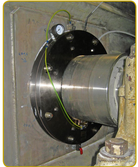
AHS INSTALLED ON A LARGE RIBBON BLENDER
