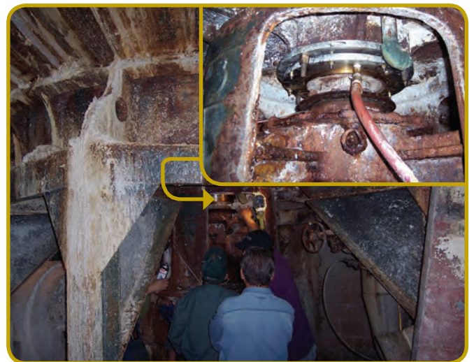
13 IN. (330MM) EA TYPE-1 SEAL MOUNTED ON A BLACK CLAWSON PAPER PULPER.
