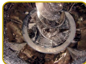
13 IN. (330MM) EA TYPE-1 SEAL MOUNTED ON A BLACK CLAWSON PAPER PULPER.
