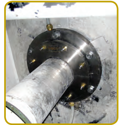
4 15 / 16 IN. EA TYPE-1 SEAL MOUNTED ON A SHEETROCK MUD MIXER.
