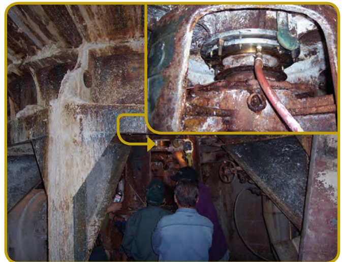
13 IN. (330MM) EA Type-1 SEAL MOUNTED ON A BLACK CLAWSON PAPER PULPER.
