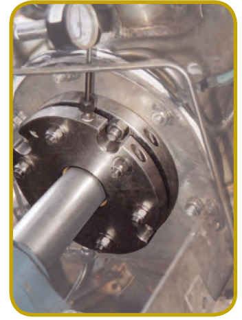
EA TYPE-2S SEAL ON A CONVEYOR WITH A 3"/75MM SHAFT
