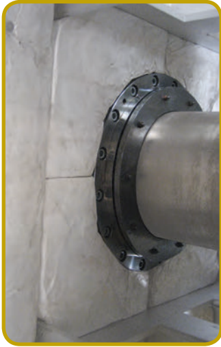
EA TYPE-2S SEAL ON A POLYMER DRYER WITH A 12.4"/315MM SHAFT
