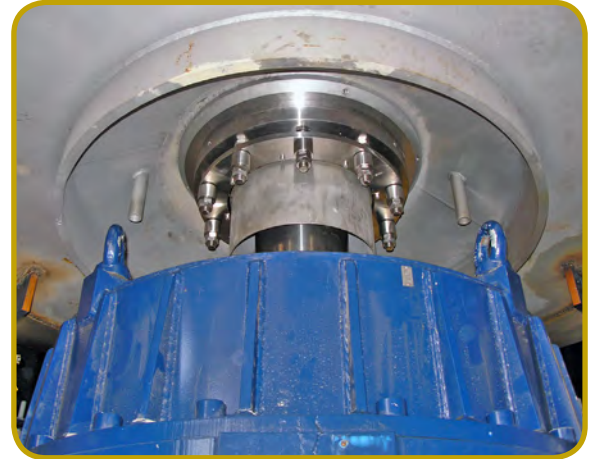
SPLIT EP TYPE-1 ON A PULPER WITH A 415MM SHAFT PROCESSING RECYCLED OFFICE PAPER.
