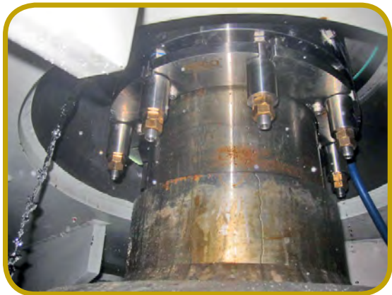
SPLIT EP TYPE-1 ON A PULPER WITH A 280MM SHAFT, PROCESSING OCC.
