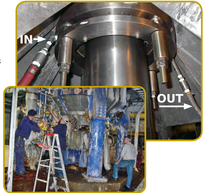
SPLIT EP TYPE-1 SEAL ON A BOTTOM ENTERING, 300MM, HI-CON PULPER
