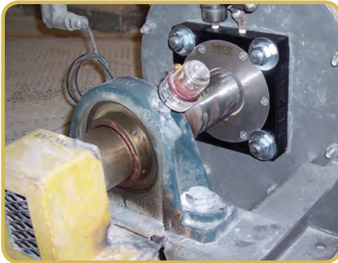
3" HBZ4W4A300 SEAL, INSTALLED ON A HORIZONTAL GYPSUM FEEDER
