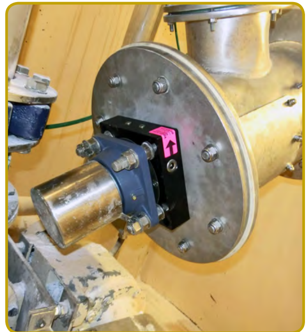
HCZ1W4A157 SEAL INSTALLED ON A 40MM SHAFT ON AN INCLINED SCREW CONVEYOR.
