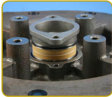
CHECKING FOR FIT IN A ROTARY FEEDER
