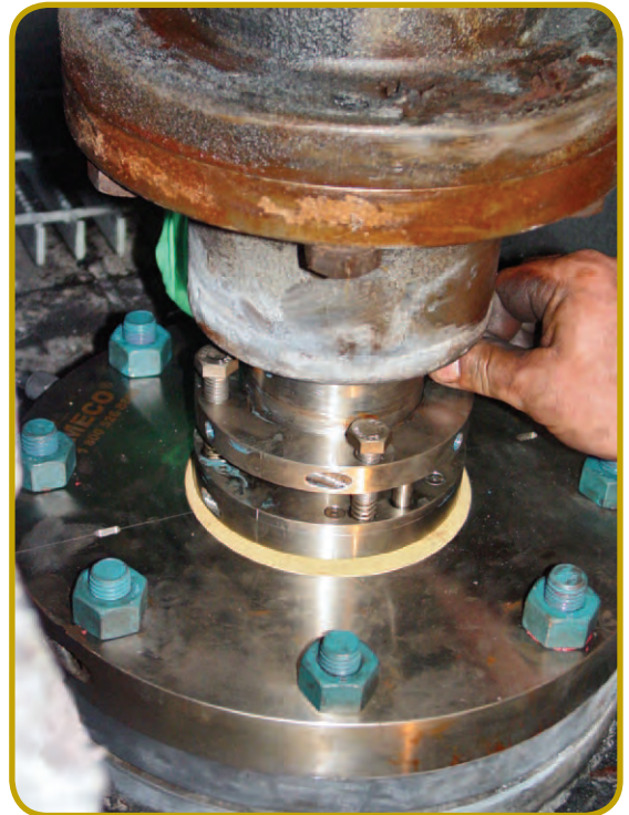
3.5" OFS Type-1 INSTALLED ON A TOP-ENTRY AGITATOR CONTAINING VOLATILE ORGANIC COMPOUNDS (VOCs).
