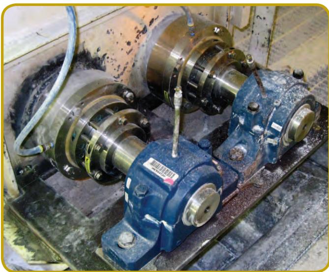
TWO 5" OFS Type-1 SPLIT SEALS INSTALLED ON A HORIZONTAL PADDLE MIXER CONTAINING FINE MINERALS
