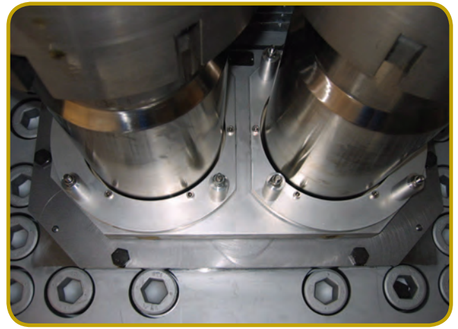
DUPLEX MECO SEAL ON COPERION ZSK-380 EXTRUDER
