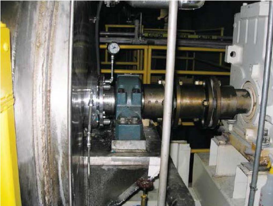
An EP seal (left) from MECO is shown mounted on the drive end of the dryer.
