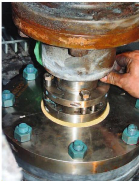
Figure 1. 3.5” OFS Type-1 installed on a top-entry agitator containing volatile organic compounds (VOCs). Source: MECO Seals
