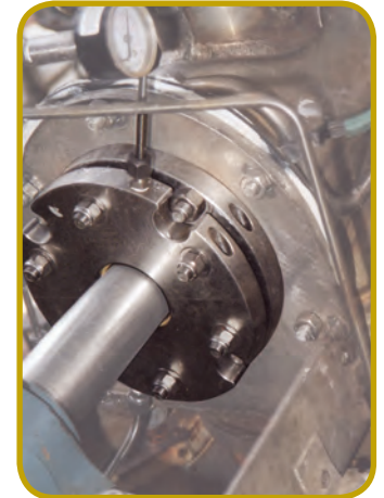
EA TYPE-2S SEAL ON A CONVEYOR WITH A 3"/75MM SHAFT.
