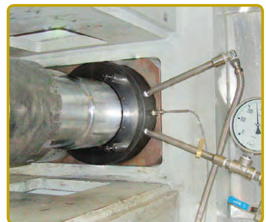
SPLIT MECO EP TYPE-2 SEAL ON A 8.7"/220MM SHAFT.
