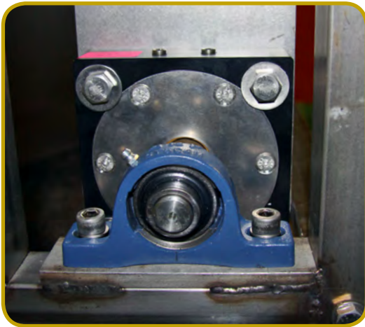
HCZ1W4A119 SEAL, INSTALLED ON A 30MM SHAFT ON A SUGAR MILL.
