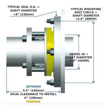
Figure 2. A built-to-order OFS Type 2 custom designed seal. Source: MECO Seals
